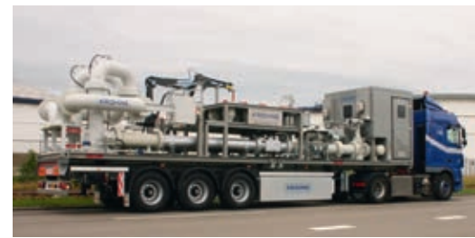
Mobile master metering system
