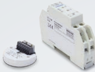
OPTITEMP TT 11 C OPTITEMP TT 11 R Analogue, adjustable 3-wire transmitters for Pt100 or Pt1000 with voltage output
